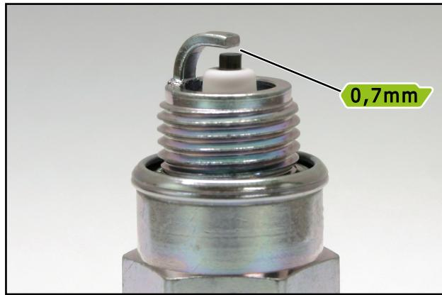
Inspect the condition of the spark plug frequently to check if the engine combustion is correct.
