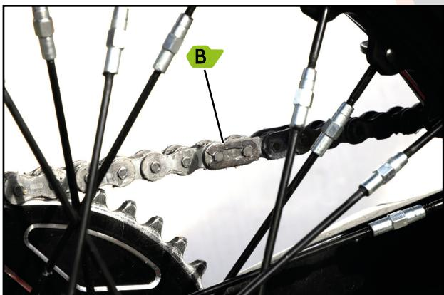
If the chain is renewed, remember that the fastening clip must be placed in the opposite direction to the travel, as indicated in the photo (B).
