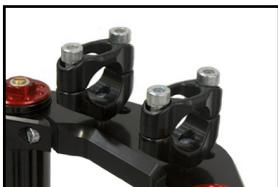
Modifying the handlebar clamps anchor to the plate with two positions available allows you to move the handlebar closer or further away.
