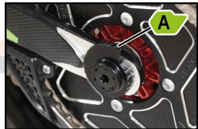
The tension should be adjusted by loosening the axle nut and turning the wheel axle with an 8 Allen key until the desired tension is achieved.
